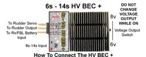
Connect the labeled (1) port on the BEC to the Rx/FBL Battery In port. Connect the labeled (2) port on the BEC to any empty channel on the Rx/FBL. If using a Rudder Servo that requires 5v, connect (2) on the BEC to the Rx/FBL Rudder out port, then connect Rudder Servo to the labeled 5v port on the BEC.
